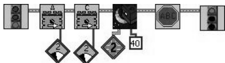
Figure 1. A RoboLab program that tells the robot to go forward until the light sensor reads a value less than 40; then stop. "Modifiers" hang down from the main control loop, which moves horizontally across the diagram, and indicate speeds, thresholds and port connections.
