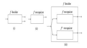
Figure: (i) a decider, (ii) a recognizer, and (iii) a decider built out of two recognizers
