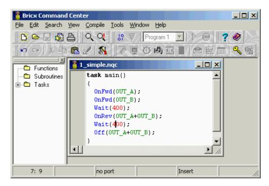
The interface looks like a standard text editor, with the usual menu's, and buttons to open and save files, print files, edit files, etc. But there are also some special menus for compiling and downloading programs to the robot and for getting information from the robot. You can ignore these for the moment.
