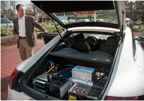
Graduate research team leader Chris Gerdes shows off the systems carried onboard the autonomous car, a modified Audi TTS.
