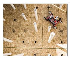
Robots are being trained to map spaces using their sensors. This robot travels through a simulated "wooded area" that has uneven terrain and randomly placed PVC pipes as "trees." It sends back data to researchers who use mapping algorithms to create a map.
