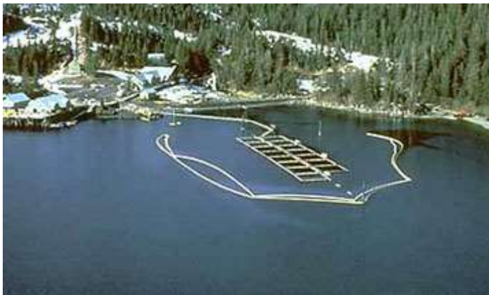
Boom surrounds a set of floating net pens at a salmon hatchery in Prince William Sound, Alaska, to protect the pens from oil spilled from the Exxon Valdez.
