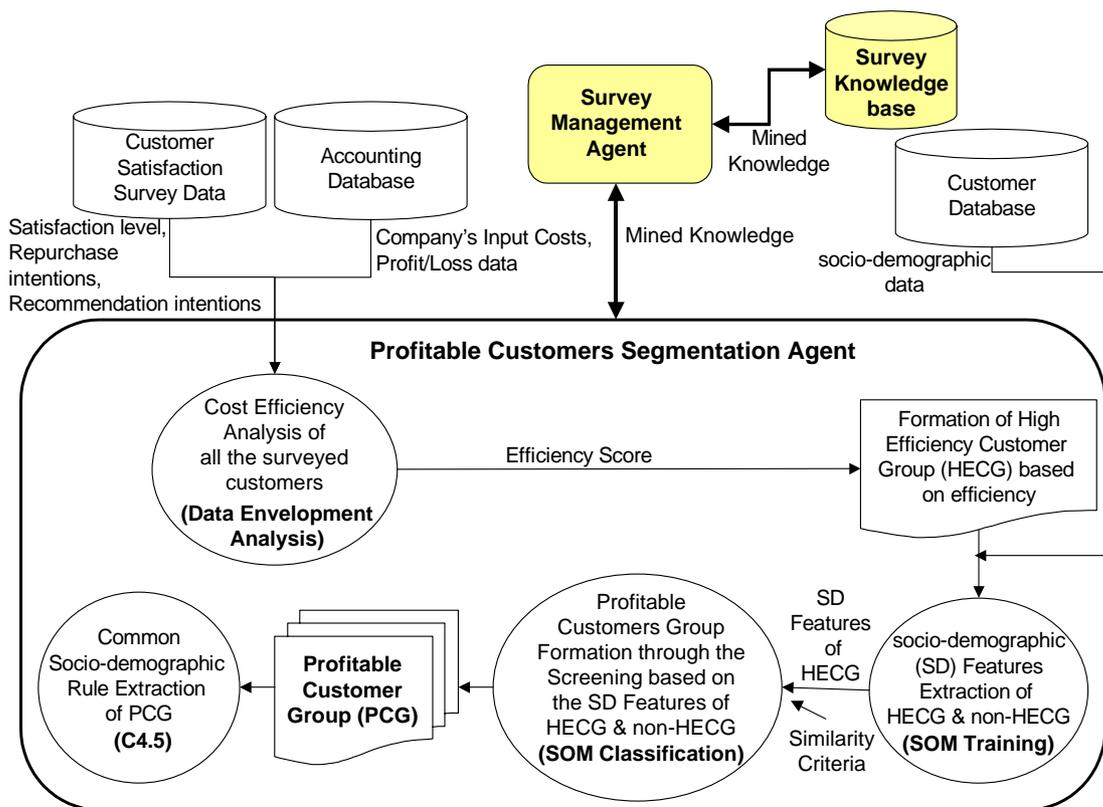
Fig. 2. Profitable customers segmentation process in PCS agent.
