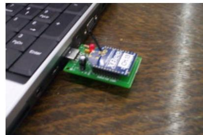
Ch13 XBee dongle
