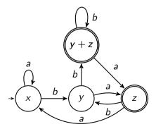
Language  $L=(a+b)^*b(a+b)$ . Second from last letter is b. Four states. Initial state given by the empty word  $q_{\rm in}=x$ . Accepting states  $Q_t=\{z,y+z\}$ . The states z and y+z correspond to the words  $(a+b)^*ba$  and  $(a+b)^*bb$ , respectively. Notation y+z comes from relation to  $\mathbb{B}$ -modules. Regular language: one recognized by an FSA.
