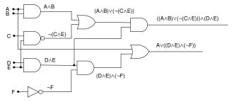
A logical circuit with 6 inputs and 2 outputs.
