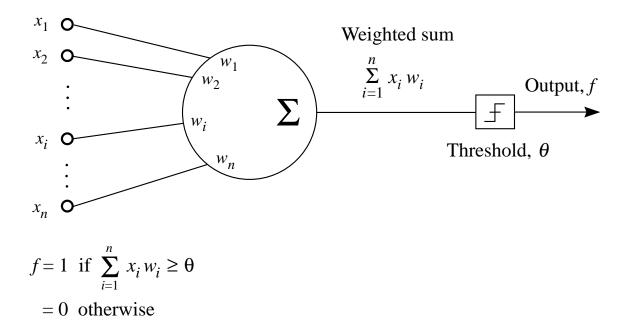
• The Boolean functions that can be computed using a TLU are called *linearly seperable* functions.
