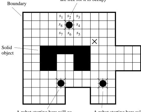
A robot starting here will go counterclockwise around the outside boundary of the object A robot starting here will go clockwise around the inside of the outer boundary
