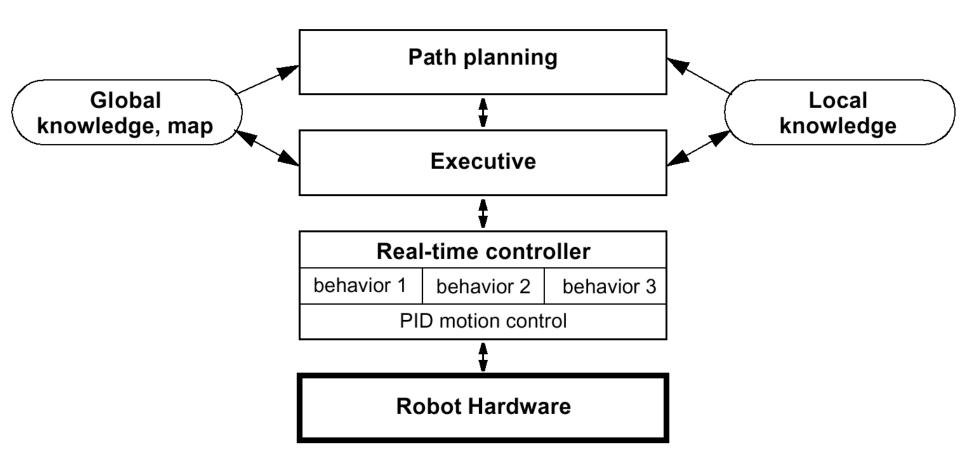
• Planner is triggered when needed: e.g. blockage, failure
