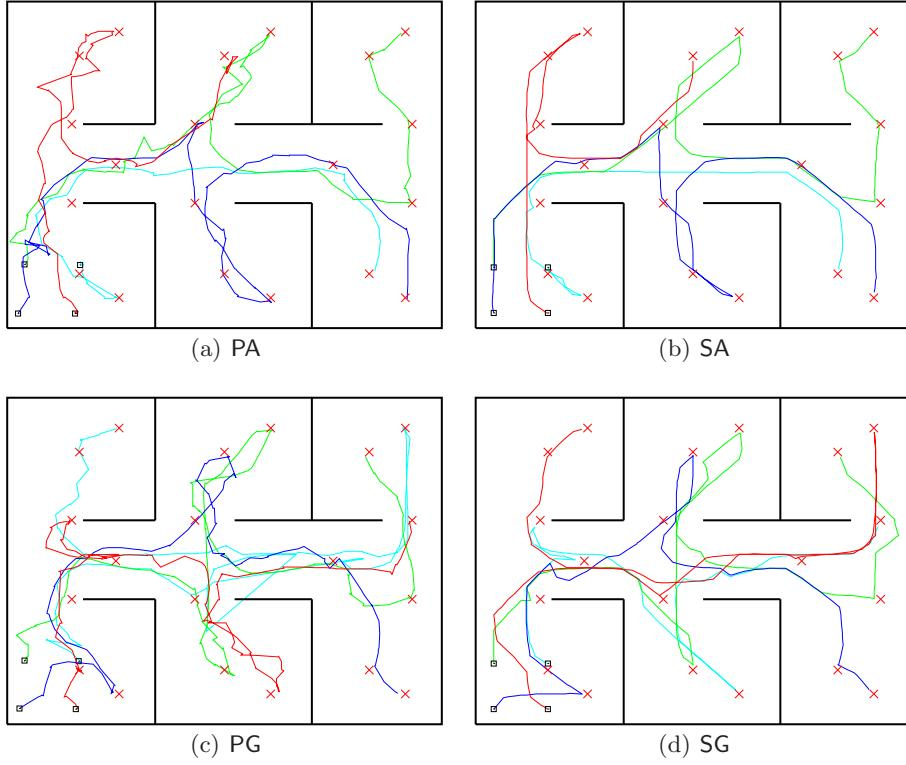
**Fig. 8.** Robot trajectories in the physical (left) and simulated (right) environments, for scenario a, using task allocation by simple auction (top) and greedy-taxi (bottom) mechanism.
