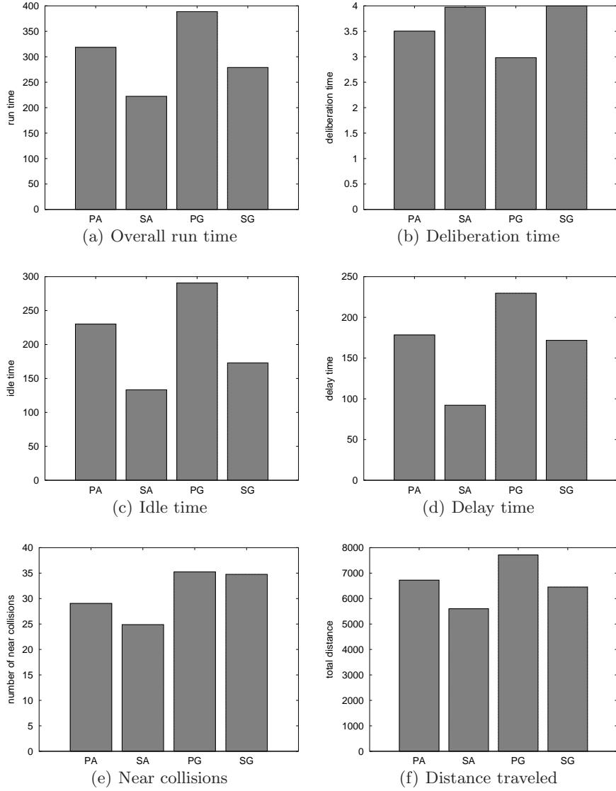
**Fig. 5.** Combined results for all scenarios. Values for each metric distinguish between the physical (P) and simulated (S) experiments, and between the simple auction (A) and greedy-taxi (G) task allocation.
