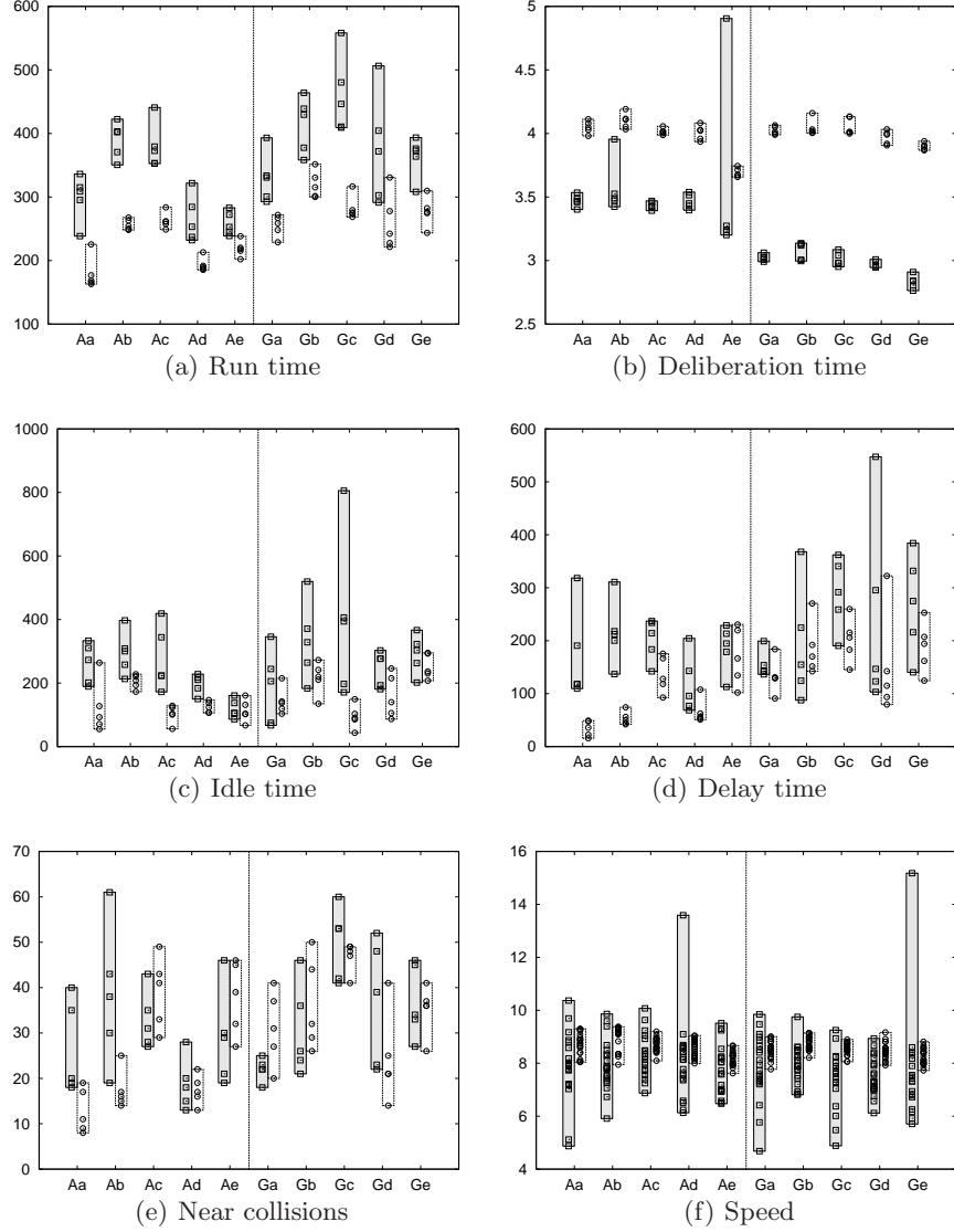
**Fig. 6.** Results from individual scenarios. We compare the range of values measured in the physical and simulated environments. Results for the physical robots are enclosed in grey boxes; results for the simulated robots are enclosed in white boxes. We distinguish between simple auction (A) and greedy-taxi (G) task allocation, for each of the five different scenarios, labelled a through e.
