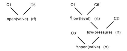
The impasse may be resolved since Yopen(value) is deduced with rough truth value rt a higher truth value than that with which the conclusion open(valve) is reached. The system can thus conclude that the valve should not be opened.
