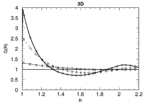
FIG. 2. Comparison of MC three-dimensional data to the results of Barker and Henderson.  $\rho=0.20$ ...MC  $\square$ ;  $\rho=0.60$ ...MC  $\triangle$ ;  $\rho=0.80$ —MC  $\circ$ .
