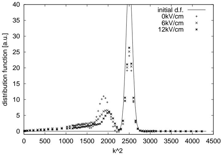
**Fig. 4.** Solutions  $kf(r, k, t)$  for  $r = 0$ ,  $k \in (0, Q)$  and evolution time  $200fs$ . The electric field is 0,  $6kV/cm$  and  $12kV/cm$ .
