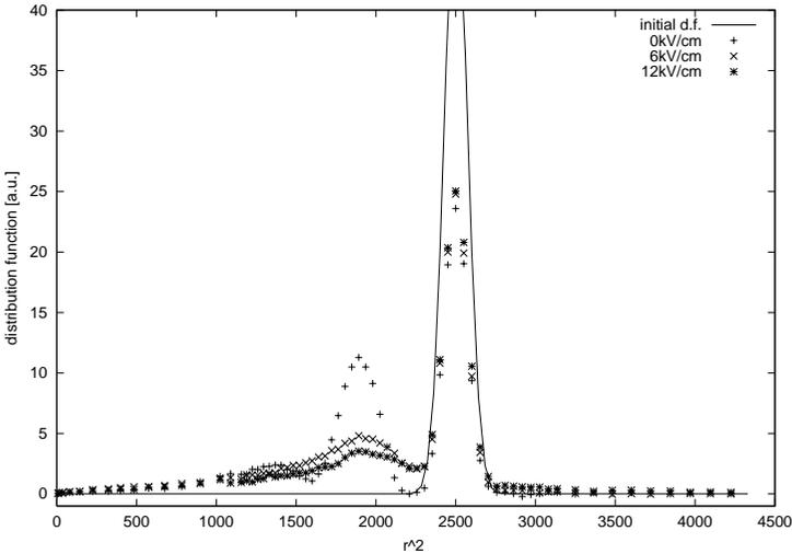
**Fig. 5.** Solutions  $rf(r, k, t)$  for  $k = 0$ ,  $r \in (0, Q)$  and evolution time  $200fs$ . The electric field is 0,  $6kV/cm$  and  $12kV/cm$ .
