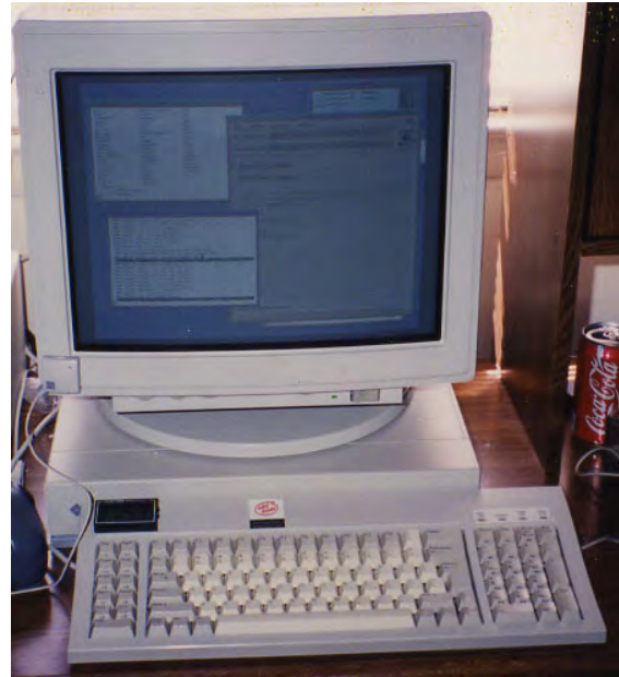
Sun SPARCstation 1+ from the early 1990s, with a 25 MHz RISC processor
