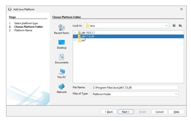
Then select the path where jdk1.7.0\_80 is installed, such as C:\Program Files\Java\jdk1.7.0\_80 then press Next.
