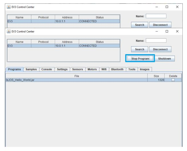
You can stop a program by pressing **Stop Program**. If the robot is not connected to the computer, you can force stop it by holding **ENTER** (center button) and pressing the **DOWN** button.
