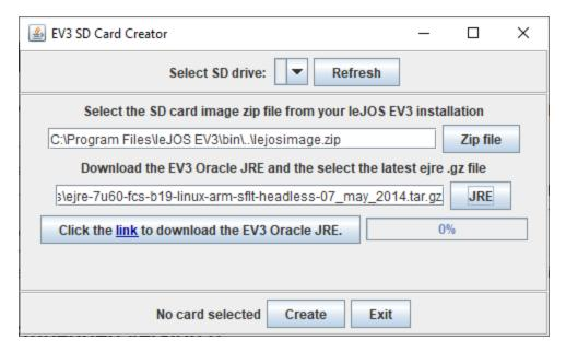
Make sure to select the SD drive from above and then press on **Create**. It will open a terminal and take some time to install. If you installed the incorrect JRE file, you will get an error when turning on the robot.
